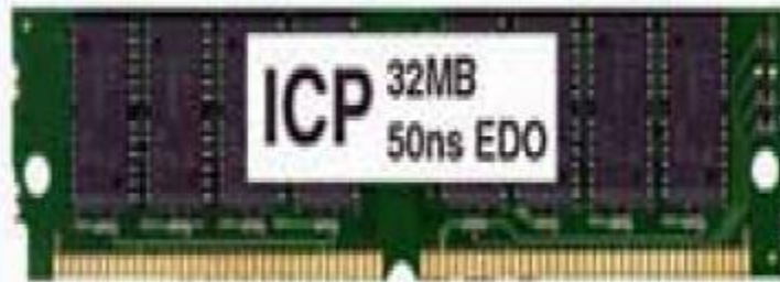
SIMM72 Single In-line Memory Module
