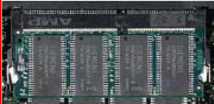
SO DIMM Small Outline Dual In-line Memory Module
