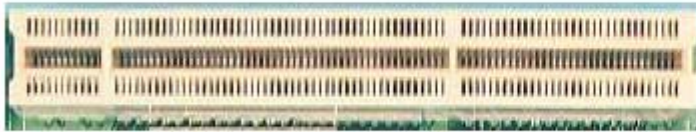
PCI 64bit 3.3V Peripheral Component Interconnect
