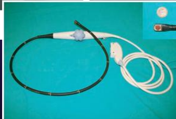
Figure 6.39 Transesophageal transducer for cardiac imaging. This transducer is swallowed by the patient and makes ultrasound images of the heart from within the esophagus. (Courtesy of the Department of Cardiology.)
